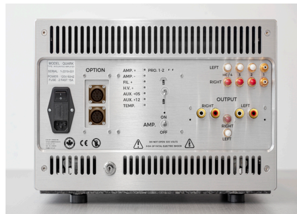
Rear view: A lock secures access to the rail system and the inside of the enclosure.
